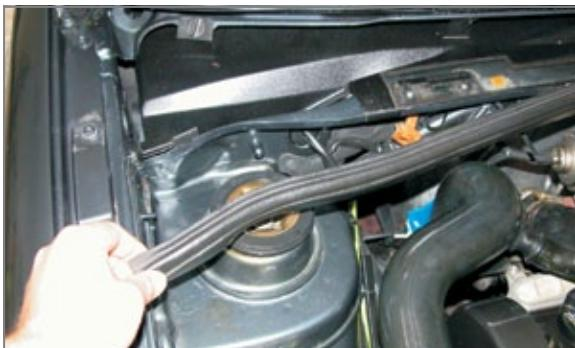
**EN** Remove the rubber seal
