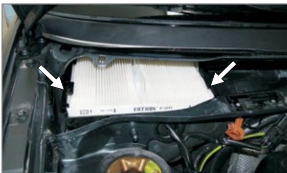
**EN** Unlatch the filter from its socket
