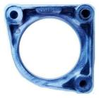
On the first generation 2.3 and 2.8JTD engine Fiat used on the Marelli/Denso: 63114014 and Bosch: 0001218159, 0001223013 0986017020, 0986018960 starters an adaptor flange. The Fiat number of the flange: 1327137080, 1327138080, 5978701
